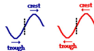
An incident wave and a reflected wave can be thought of as merely a repeating pattern of crests and troughs.
